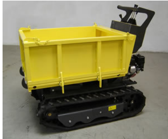
Figure 6. The minidumper used for mounting the ladder
