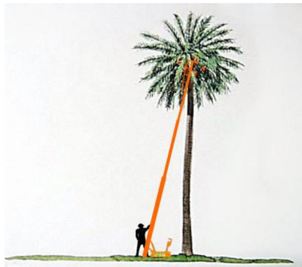
Figure 8. Draft of the equipment positioned to service a date palm bearing fruits at a height of about 10 m. The figure shows the proportions within the sizes of the different components
