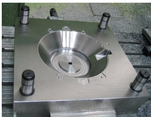
Figure 2. Particular of the die for the production of the bottom of the guard
