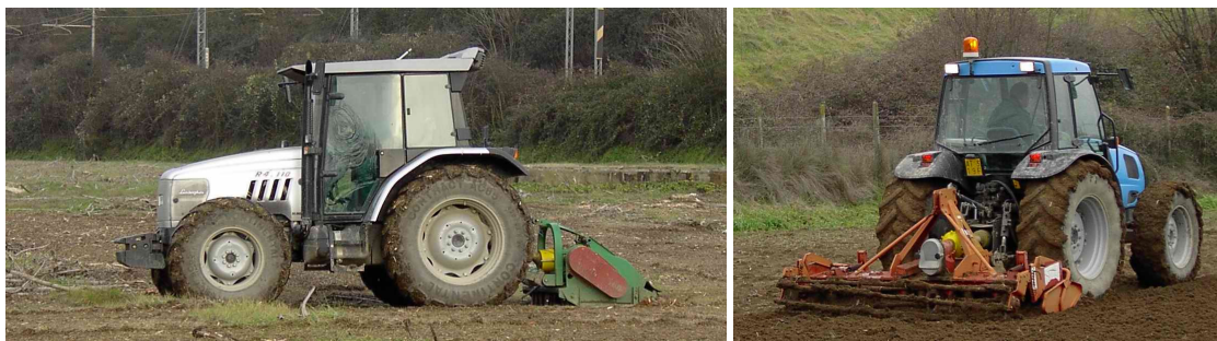
Figure 4. The prototype has been tested under different working conditions such as the chopping of poplar residues with a stump grinder (left) and soil refinement with a rotary harrow (right)
