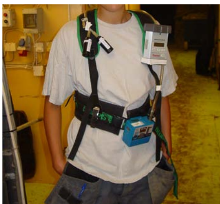
Figure 1. Instrument used for the personal sampling (a portable air pump that was connected with two sampling filters and the DataRAM).
