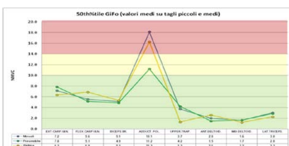
Figures 6-7. Diagrams of MVC% 50th percentile of the two subjects (TeMo: female code and GiFo: male code) obtained by calculating the average values of pneumatic and manual scissors as compared with electric scissors by averaging small and medium cutting values. The diagram highlights the values recommended by Jonson B., 1978 through coloured bands on the background: green = area below limit (<10MVC%), yellow= border area (10-14 MVC %), red= area above limit(>14MVC%).
