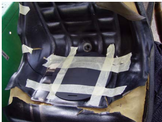
Figure 3. The triaxial seat transducer.
