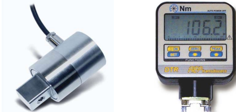
Fig. 1 – The torsionmeter and the digital torque indicator
