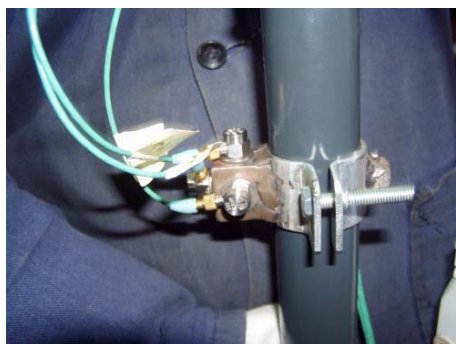
Figure 2. Positioning of the accelerometers on the bar. Figure 3. Reference axes for vibration measurement.
