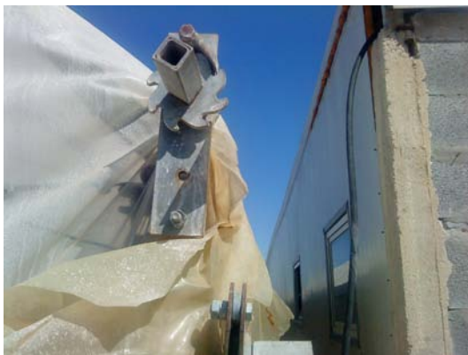
Fig. 2 - The wrapping groups: the “rosetta” and its 8 curved points, the hollow end of the rod, the blocking systems with the hinged mobile tooth; the whole rod is not visible here
