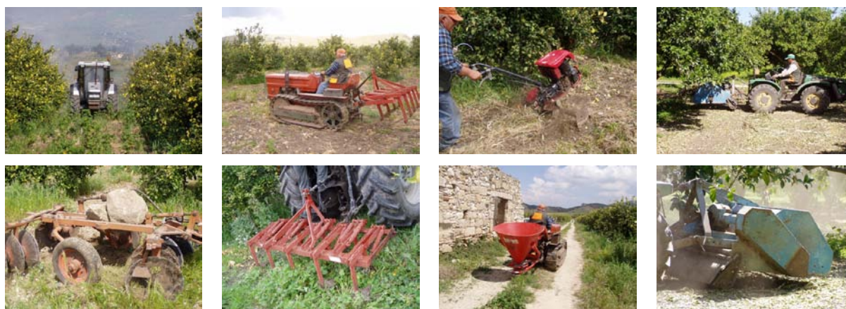
Figure 1. Tractors and operating machines used for the experimental tests (from top to bottom, from left to right): wheeled tractor with cab; tracked tractor; rototiller; wheeled tractor without cab; disk harrow; tooth harrow; fertiliser; pruning triturator.
