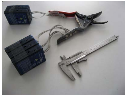
Fig.1: Shear with sensors connected to wireless transmitters
