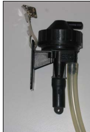
Figure 2. SKC cyclone for respirable fraction
