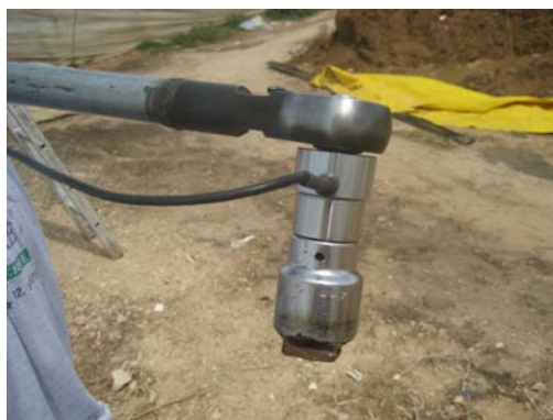
Fig. 3 - The long lever used for stretching the film, with the pawl, the torsionmeter and the square key to insert in the hollow end of the rod
