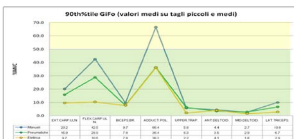
Figures 8-9. Diagrams of MVC% 90th percentile of the two subjects (TeMo: female code and GiFo: male code) obtained by calculating the average values of pneumatic and manual scissors as compared with electric scissors by averaging small and medium cutting values. The diagram highlights the values recommended by Jonson B., 1978 through coloured bands on the background: green = area below limit (<50MVC%), yellow= border area (50-70 MVC %), red= area above limit(>70 MVC%).
