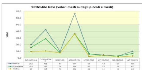
Figures 8-9. Diagrams of MVC% 90th percentile of the two subjects (TeMo: female code and GiFo: male code) obtained by calculating the average values of pneumatic and manual scissors as compared with electric scissors by averaging small and medium cutting values. The diagram highlights the values recommended by Jonson B., 1978 through coloured bands on the background: green = area below limit (<50MVC%), yellow= border area (50-70 MVC %), red= area above limit(>70 MVC%).
