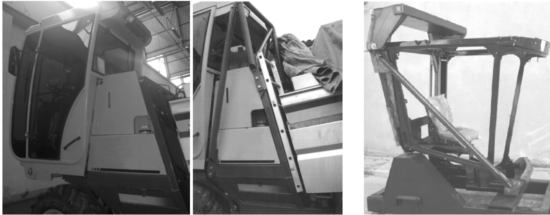
Figure 1. Tested ROPSs. (a) CASE 1 (b) CASE 2
