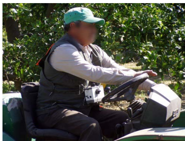
Figure 3. Positioning of the dust monitor during the experimental tests.
