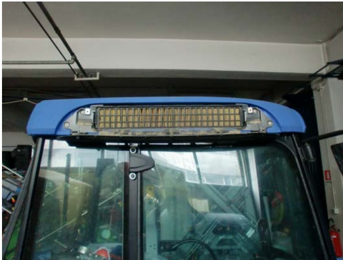
Figure 4_ Particular of cabin filter housing
