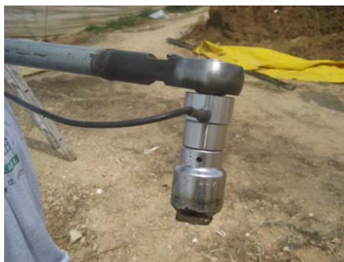
Fig. 3 - The long lever used for stretching the film, with the pawl, the torsiometer and the square key to insert in the hollow end of the rod
