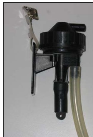
Figure 2. SKC cyclone for respirable fraction
