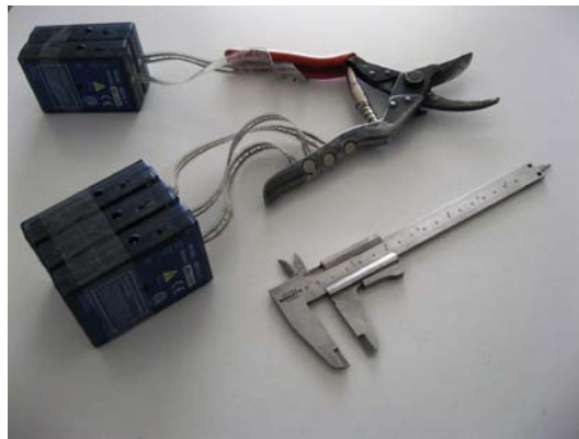
Fig.1: Shear with sensors connected to wireless transmitters
