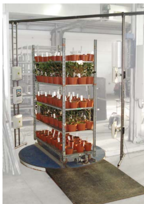
Figure 3. Dynamic multiple reading of 129 potted plant identified by means of plastic label UHF transponder during wrapping process before shipping.
