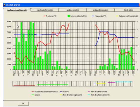
Fig. 6. Outputs by the model: external temperature, power required, set temperature, diffuse radiation.
