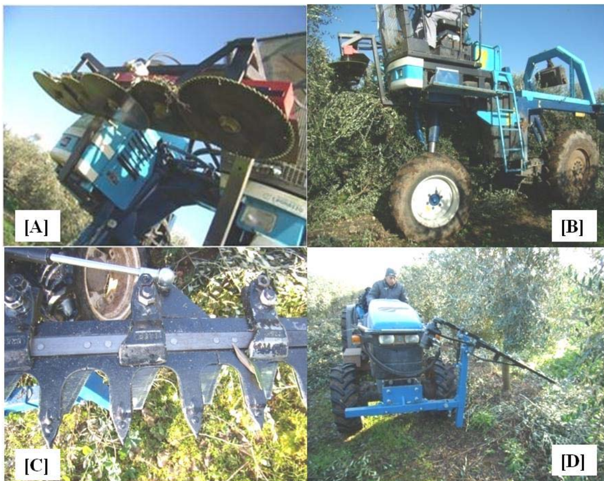
Figure 1. Pruners employed for interventions of topping at height 2,20 m from the ground in an olive grove of the FS 17 variety (7 th year from the planting) : [A]- pruner risen by «BMV» with 5 disk; [B] straddle tractor «BRAUD» SB56; [C] mowing bar; [D] mowing bar mounted on the tractor.
