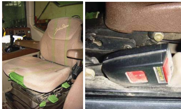
Figure 8. A seat intact, equipped with a system of retention of the driver (seat belt).
