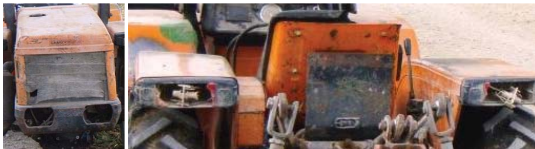
Figure 3. Example of tractor with broken lighting devices
