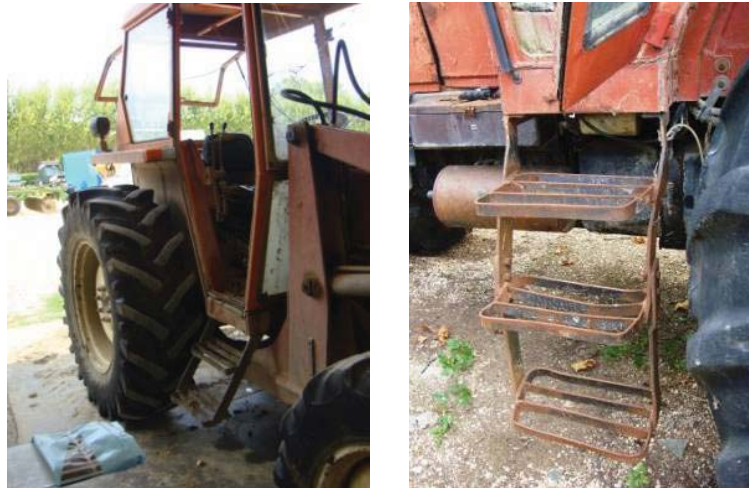
Figure 2. Left: access to the driving position without handle. Right: ladder platforms with evident corrosion and deformation
