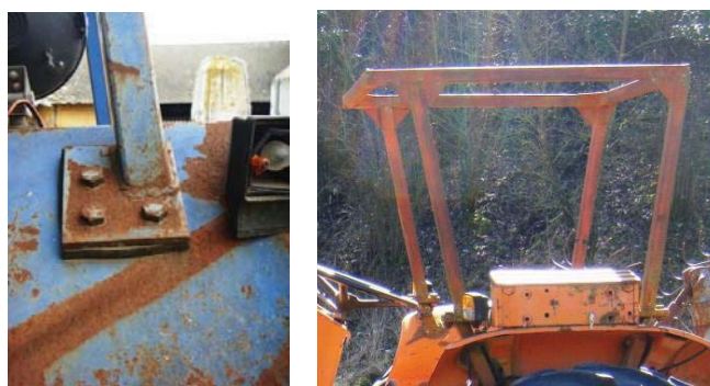
Figure 6. Left: protective frame with evident signs of corrosion in progress. Right: four-post frame without identification label. The points of anchorage to the tractor frame are in poor condition.
